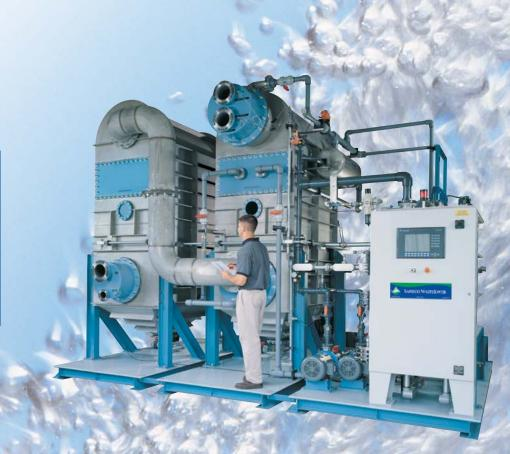
Patented Pumpless Liquid Transfer System (EVAC™) does not require feed, distillate, or concentrate pumps as do other distillation systems. This increases reliability while eliminating all problems associated with pumps, seals, impellers, and other mechanical liquid transfer components. This includes costly pump maintenance, pump replacement (and associated downtime), electrical hazards, and spare parts inventory.
